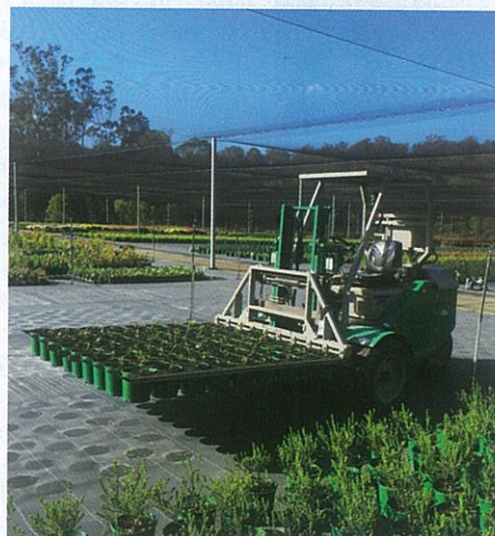
The Prins Fork is used to space pots and has meant huge savings in labour.
